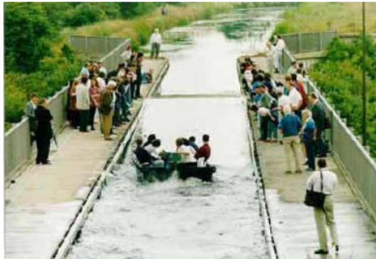
Figure 1.1: Recreation of a solitary wave on the Scott Russell Aqueduct on the Union Canal. Photograph courtesy of Heriot-Watt University [93].
