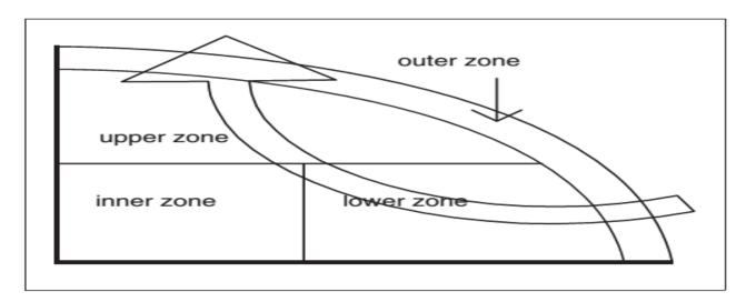
Figure 5: Cross section of a compost windrow (major zones and convection stream are indicated).
