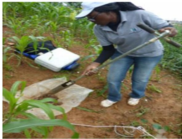
Appendix 3. Some of the laboratory apparatus used for this study. (a: GPS Map 64s Garmin; b: Auger round-tipped, iron support, handle wrench vt-66 chrom-vanadium, trowel santos 22cm, meter Stanley tylon 5m; c: Calibration solution; d: Multi 3320 meter box WTW; e & f: ICP-OES Spectrometer PerkinElmer - Model Optima™ 8300).
