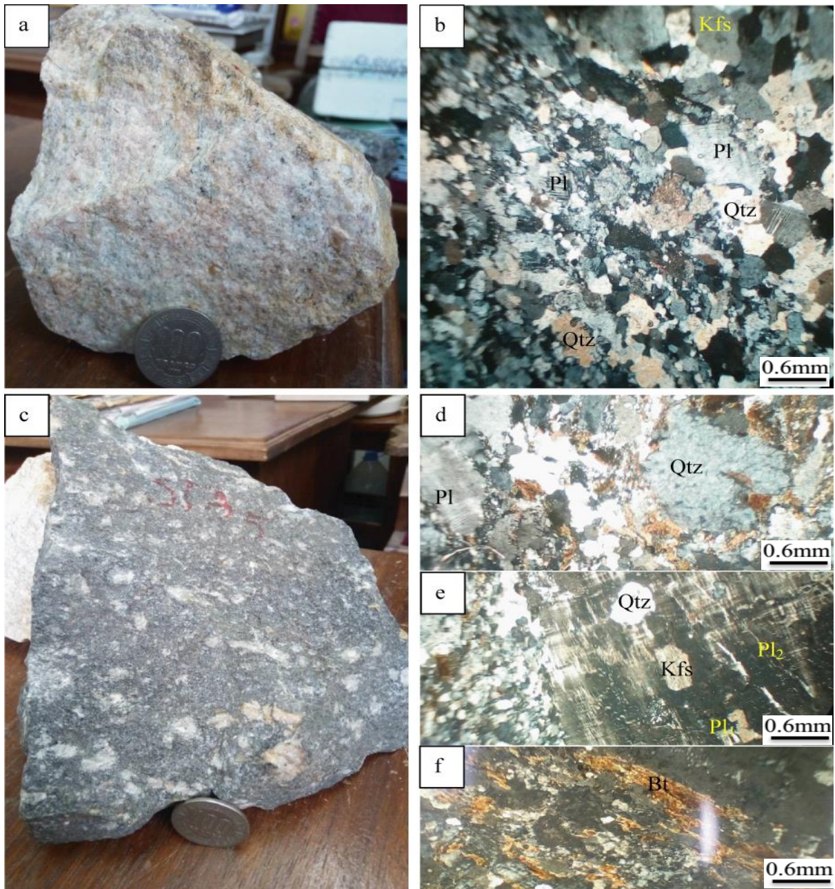
Figure 16: Granite samples from Etam: a) Hand specimen of fine grained granite; (b) Photomicrograph showing equigranular microtexture in fine grained granite; c) Hand specimen of biotite granite; d) Photomicrograph showing microtexture aspect of biotite granite; e) Phenocrystal of plagioclase containing Qtz, Kfs as inclusion, f) Preferred orientation of biotite minerals in biotite granite.
