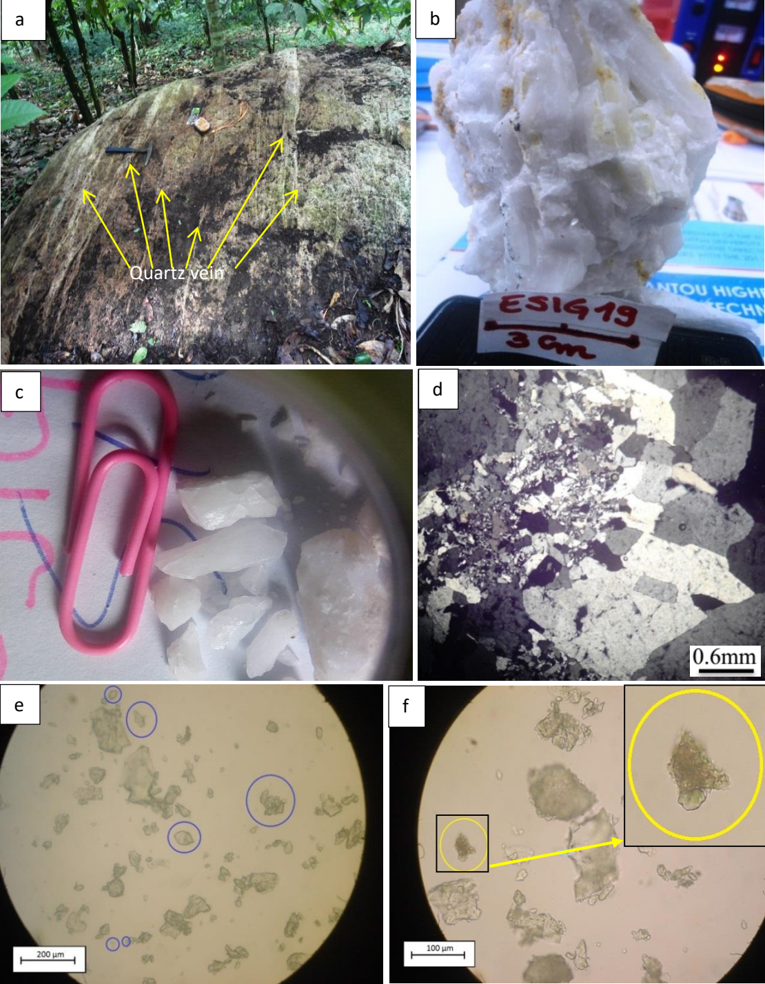
Figure 44: Field Features and petrography of the milky quartz: a) Brecciated quartzite block showing small quartz veins lenses, b) hand specimen of milky quartz clast, c) Milky quartz clast size (up to 12 cm), d) photomicrograph of milky quartz with quartz inclusion. e) Small recrystallized hexagonal quartz grain (blue circle). These grains constitute the siliceous matrix healding clasts. f) Cluster of small quartz grain contening red spot, probably iron oxide.
