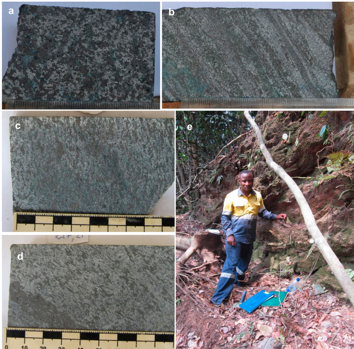
Figure 12. Various textures of foliated itabirite: (a) Foliated BIF itabirite sampled at 145 m depth from a drill hole in TNF11; (b) Unfoliated GIF itabirite (TNDF11_02, 114 m); (c) Incipiently foliated itabirite (TNDF11_02, 147,76 m); (d) Moderate to strongly foliated itabirite with S-C fabric, S-Planes dominant (TNDF11_02, 255 m); (e) Strongly foliated to mylonitic itabirite with S-C fabric, C-Planes dominant (outcrop).
