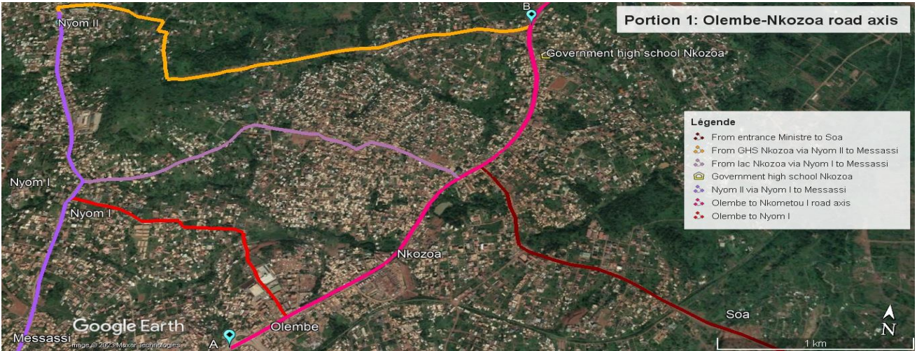
Figure 23: Portion 1: Possible locations of the new secondary roads that can be created from Olembe-Nkozoa road axis.
