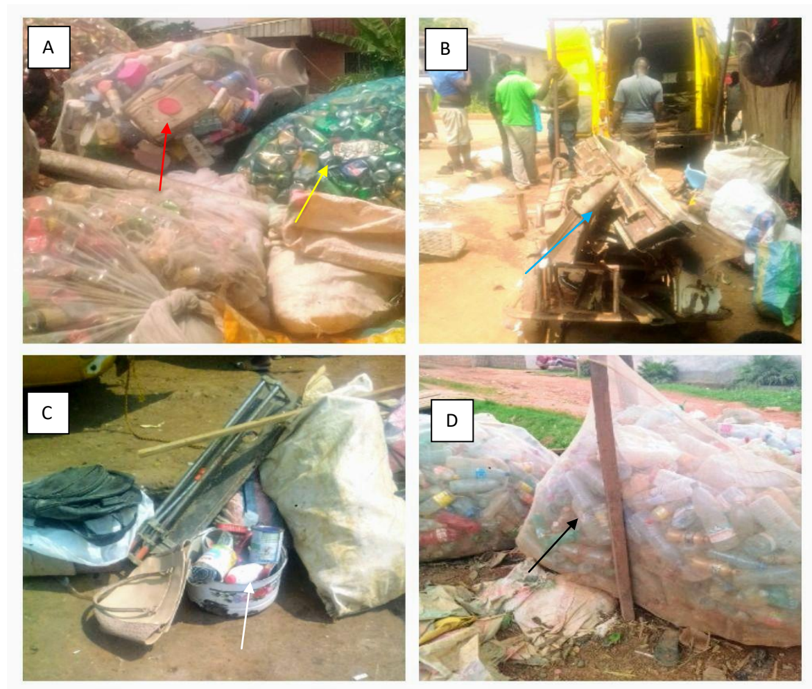
Plate 9: Sorted HDPE containers and aluminium cans (A), end-of-life vehicle scrap metal (B), tin cans(C) and PET bottles (D)
