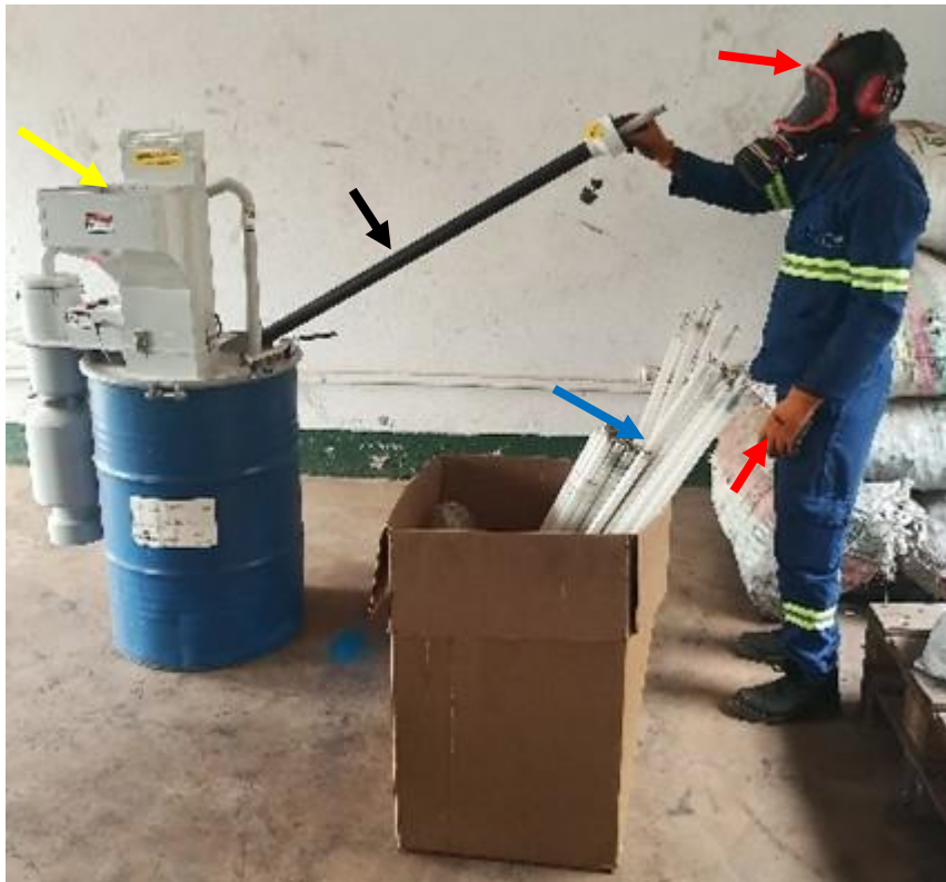
Photo 27: Treatment of mercury containing fluorescent lamps
