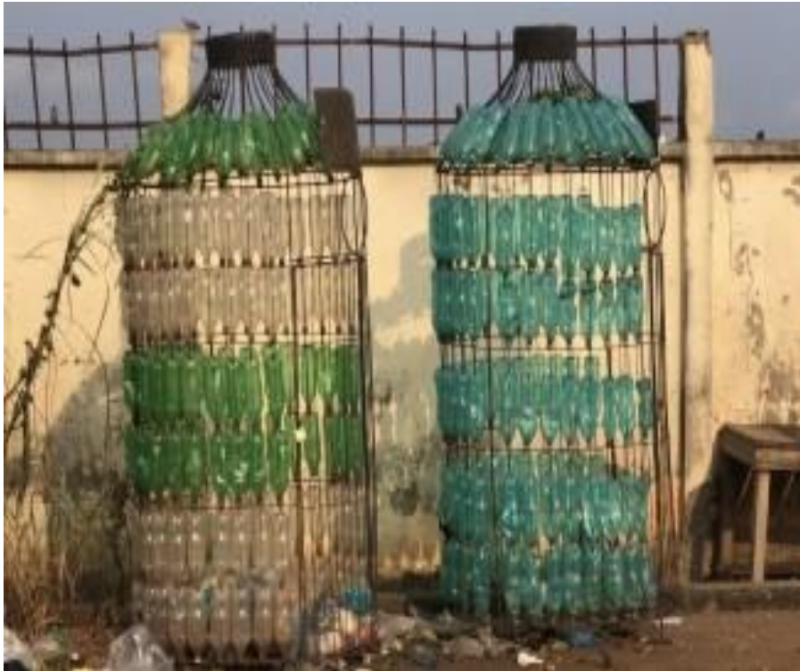
Photo 17: Plastic bottle receptacles on steel structures
