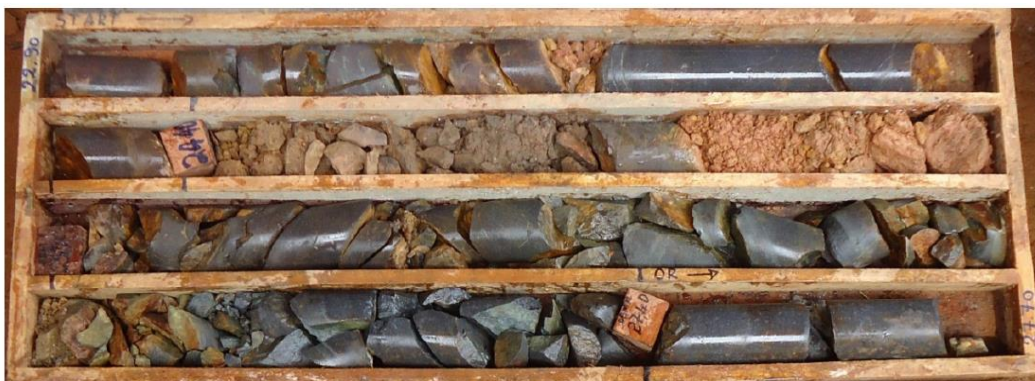
Figure 21. Brittle deformation (fracturing) in drill core, preserved in SBIF hole TH25.
