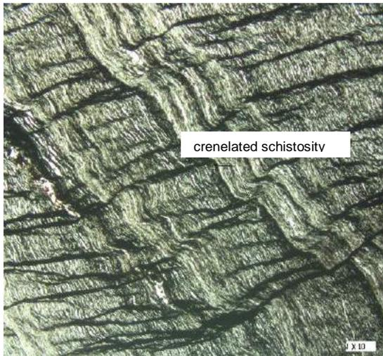
**Fig. 5.** Microphotograph showing a crenelated schistosity observed in black schists.
