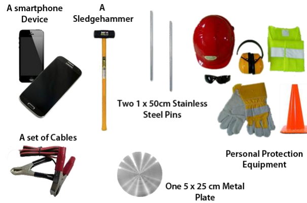
Figure 7: Survey Equipment for the ES Method
