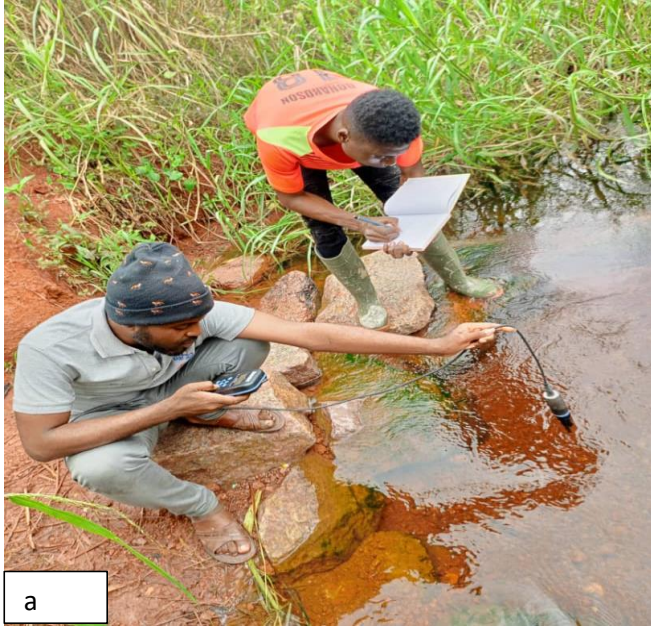
Field work and materials used to determine in-situ physicochemical quality of water at the control site along the Mongoukele (a) and on the mining site at Kambele along the Djengou watershed (b) using a multi-parameter.
