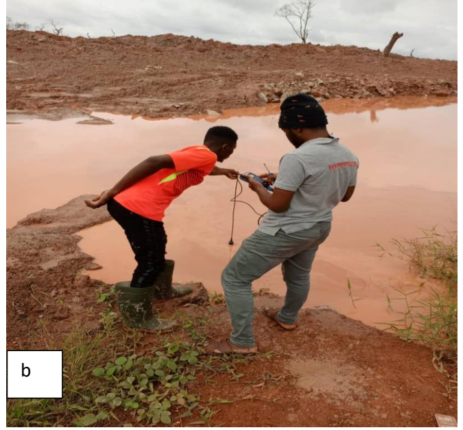
Field work and materials used to determine in-situ physicochemical quality of water at the control site along the Mongoukele (a) and on the mining site at Kambele along the Djengou watershed (b) using a multi-parameter.
