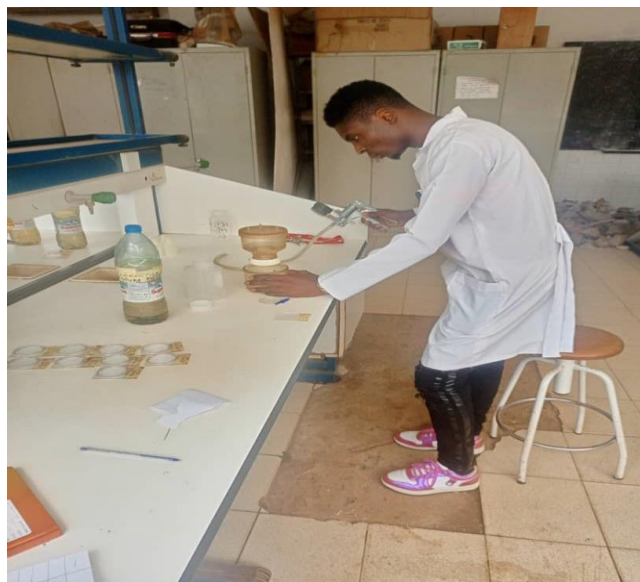
a) Determining TSS with the help of a filter (for heavy metal determination in sediment and water)
