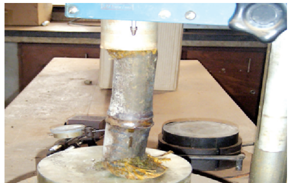
Picture. 2b Wet Specimen under the press
