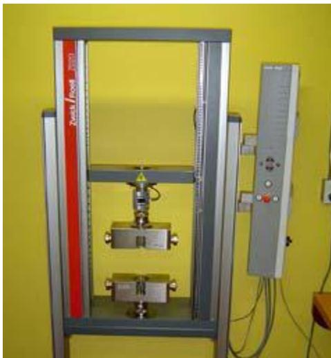
Figure 2.23: Test de traction.
