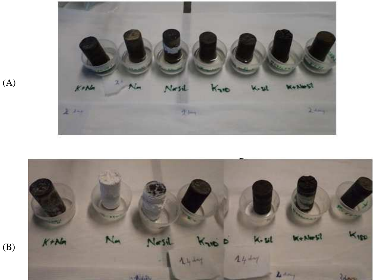
Photo 9: Specimens for efflorescence test after 2 days (A) and 14 days (B)
