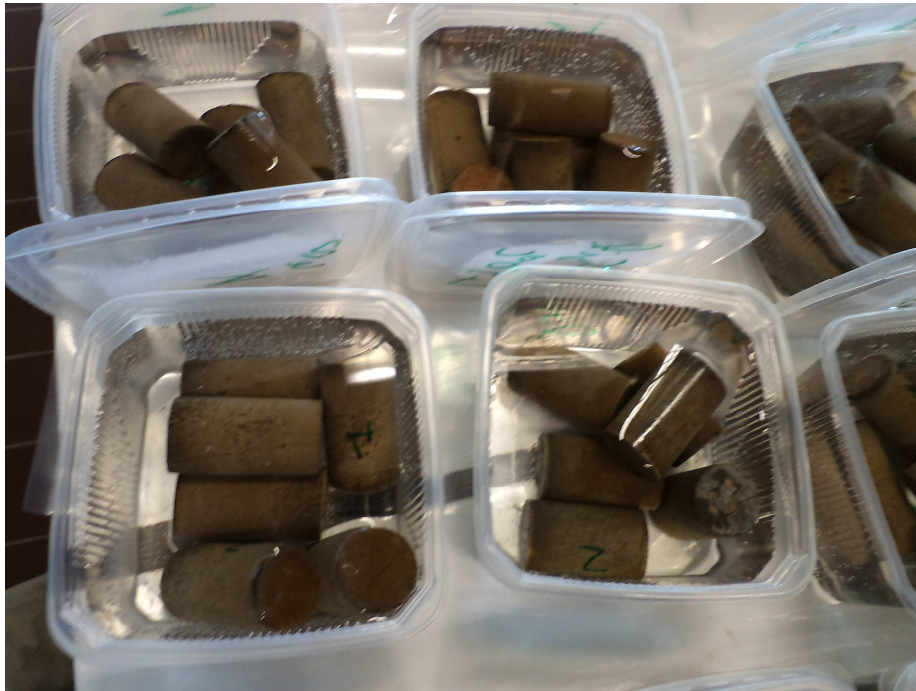
Photo 8: Specimens (Va-K, Va-K0.18, Va-KSil, Va-Na+K, Va-(Na+K)Sil, Va-Na, Va-NaSil) in immersion prior to wet compressive strength measurement.
