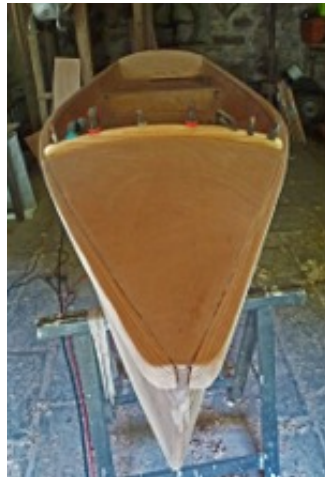
Figure 3.12 – Pose des ponts
