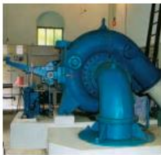
FIGURE 1.13 – Turbine Banki-Mitchell (cross-flow) [2]
