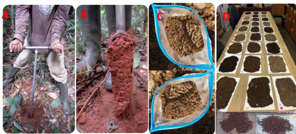
Fig. 17. Major steps to collect soil sampling in the field
