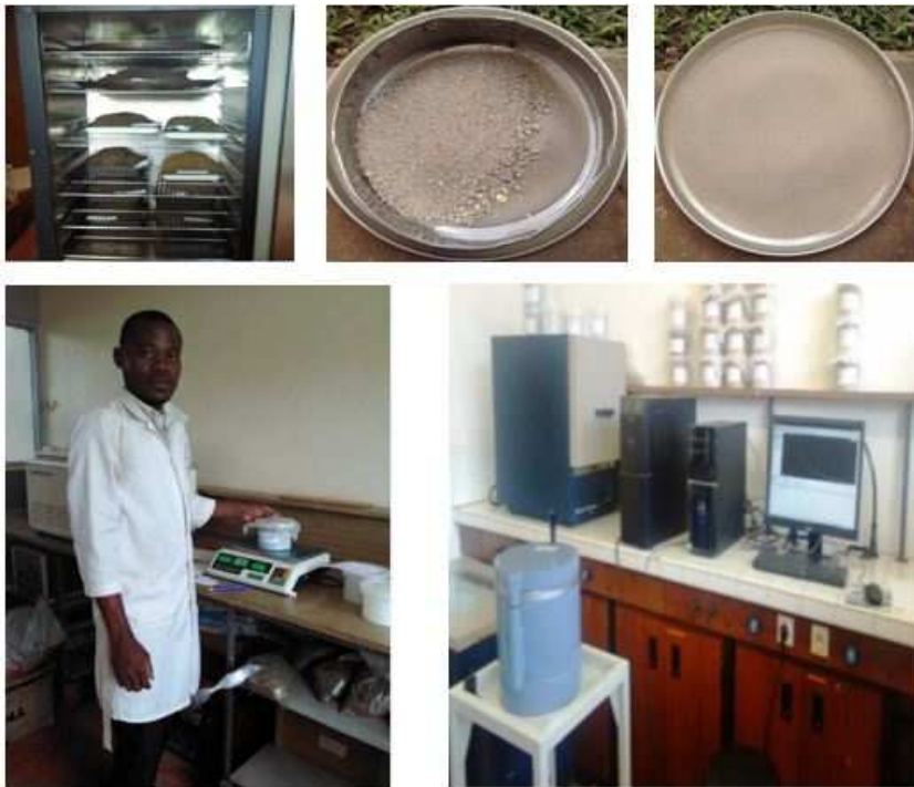
Figure 22: Sample preparation for direct gamma spectrometry.
