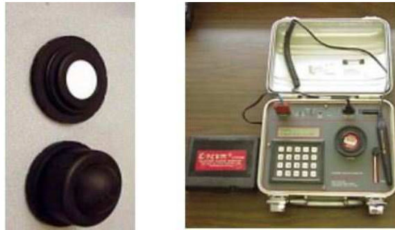
Figure 28: Electret Ion Chambers (EICs) (left) and electret voltage reader (right).
