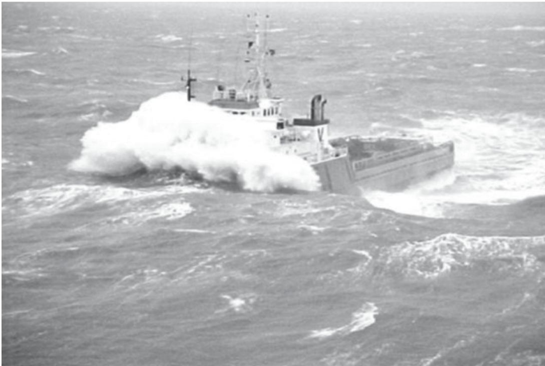
Figure 5: A "diving" into a boat. The case looks similar to the descriptions of the accident with the Taganrogsky Zaliv [53].
