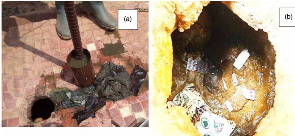
Figure 2 | Solid wastes found in the pits of the latrines investigated during FS sampling: (a) clothes and (b) a mixture of wastes in a shallow pit.
